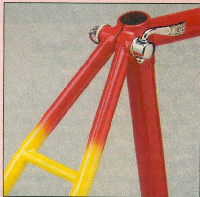
Reinforced seat collar with fillet-brazed seat-stay cluster is a Tom Ritchey trademark, and one of the frame joints he brazes.
