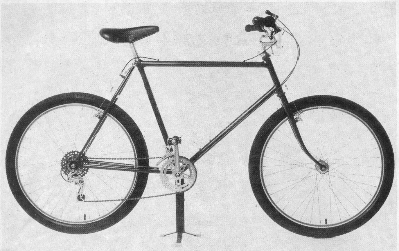
ABOVE: The Tom Richey 28 pound Mountain Bike really proves out the old adage, "The only difference between men and boys is the price of their toys". BELOW: The final drive ratios are accomplished through a Sun Tour 6-Speed cluster, Sugino Mighty Tour crankset, and a Shimano 600 front derailleur and Shimano rear derailleur.
