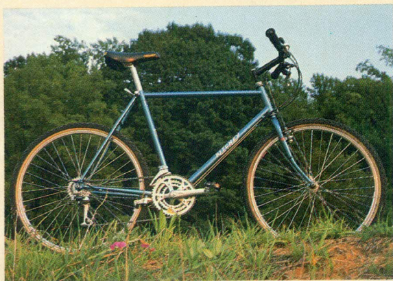
Tom Ritchey's latest creation, the Outback, uses a steep 71.5-degree head angle for a versatile bike suitable for sport riding or expedition touring on or off road.
