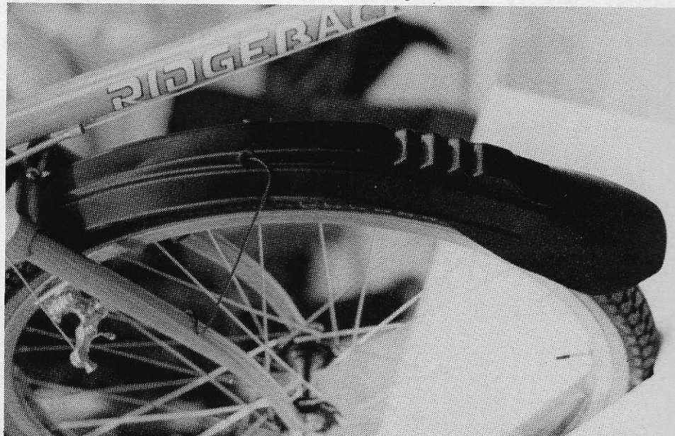
Easily removable plastic off-road fenders from Madison of England.
