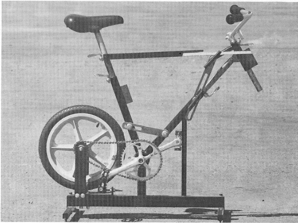
We caught this sizing machine, a Cycle Sizer from Serrota modified for mountain bike adjustment, at the Fisher factory. This is built for comfort, not for speed.
