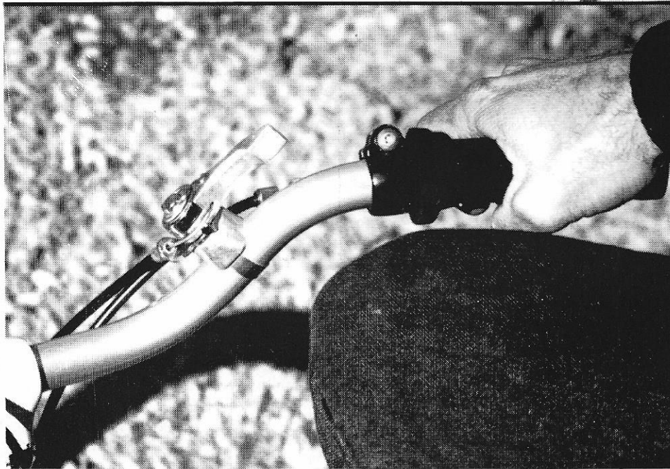
No knee knockers! Scot mounts his shifters out of the way and his brake levers downside-up to make the trials contortions as painless as possible.
