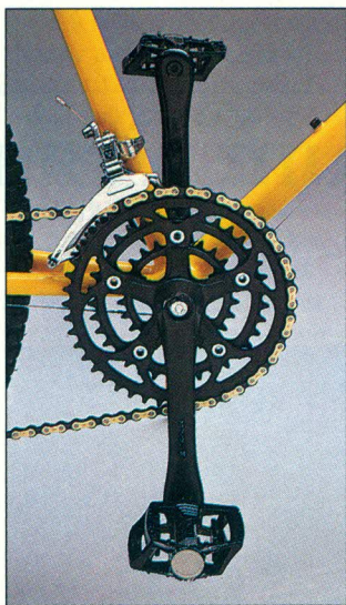
The Mt. Tam has either a Sugino AT or Takagi XT triple crankset.
