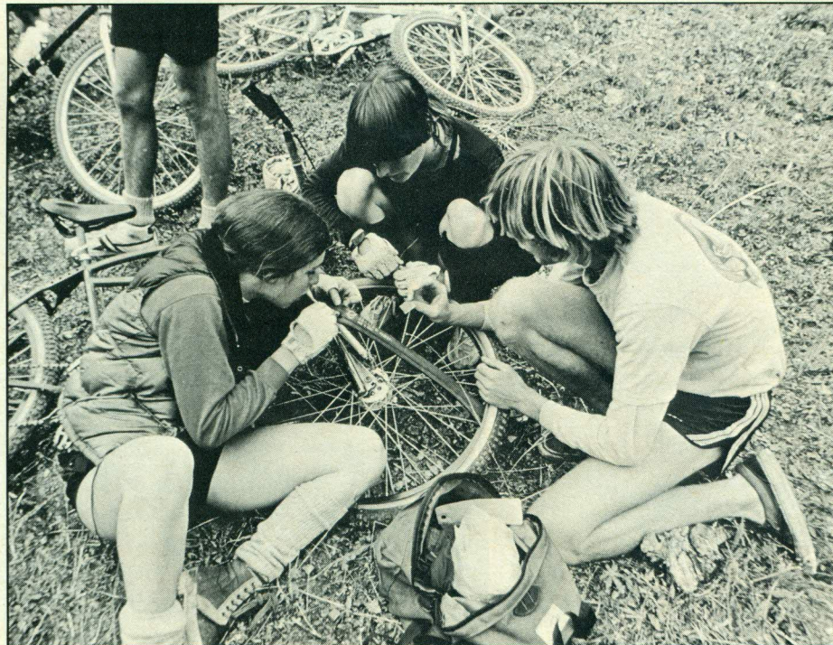
Although infrequent, flats will obviously occur, so a patch kit is absolutely necessary, and a spare tube can be handy. On this trip, six bikers got flats after riding over the same exposed nail on a horseshoe.
