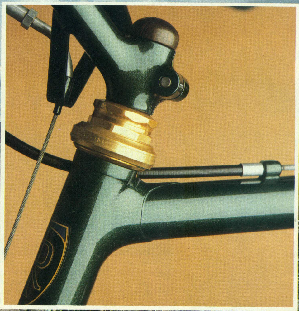
(Above) Flawless brass fillet brazing has always been a trademark of frame-builder Tom Ritchey, who built this MountainBikes Annapurna frame in his California shop. The reinforcing sleeves, sculpted to look like lugs, and the hardwood plug atop the handlebar/stem unit are additional touches. To reuse an old popular saying, "This frame has lugwork in places where other frames don't even have places!" (Left) The Trek 850's front end shows rims and hubs anodized black, to match the paint. Braking surfaces on the rims are left silver, since brake shoes wear the black anodizing off anyway. Note that the Trek, like almost all off-road bikes, uses solid axles and axle nuts instead of quick-release hubs. Solid axles are stronger than hollow quick-releases axles—a factor off-road testers have come to value. Sally Shenk Ullman photos.
