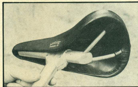
This is the lightest seat/seat-post combo we've ever seen, except maybe the old Uni-Seat. It's an Avocet seat modified by Tom Ritchey. The undercarriage, clamp, and seat post are aluminum. Total weight: 19 ounces!
